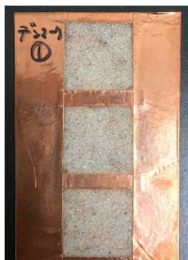
Figure 2. Powdered samples fix on a copper plate. Irradiation size was 2 × 2 cm each.
