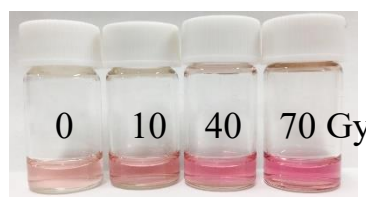
Figure 10. Absorption spectral changes (top) and sample images (bottom) of aqueous solution of 4a after \gamma irradiation.
