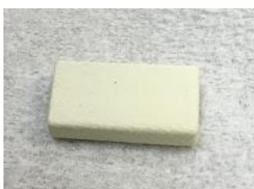
Figure 8. SUS304 with ZrO_2 film.
