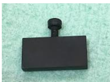
Figure 7. SUS304 with SCW oxide film.
