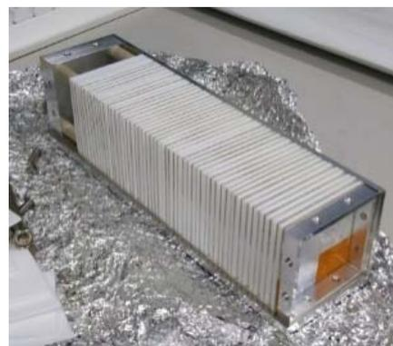
Figure 1. CR-39 stack detector.
