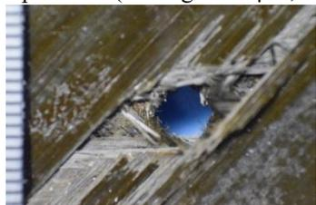
(a-2) Rear side (coating of 20  $\mu\text{m}$ , 3.11 km/s)
