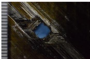
(a-1) Impact side (coating of 20  $\mu\text{m}$ , 3.11 km/s)
