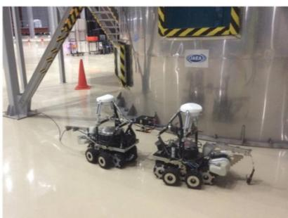
Figure 3 Demonstration of installation of a POPI seismometer around a water tank in NARREC by a specially designed robot
