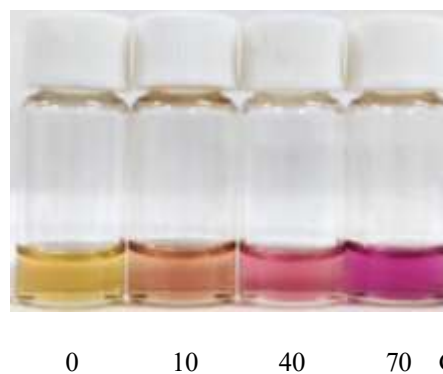
Figure 16. Images of acetone solution of 2 and X after \gamma irradiation ( [2]_0 = 0.13 mM, [X]_0 = 3.25 mM).
