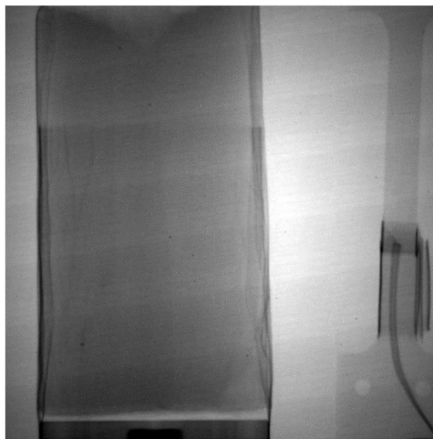
Fig.4 Neutron transmission photograph of the cylindrical shape sample and the tensile testing sample by TNRF.
