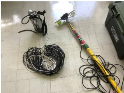
Fig. 1 Portable Water Sampler and Lighting Equipment
