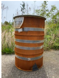
Fig.1 A drum left for 4 months for accelerated corrosion test @ JAEA.
