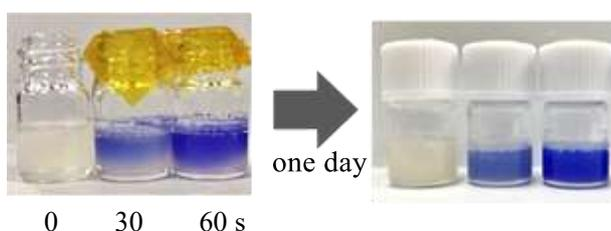
Figure 3. Image of dry dichloromethane gel of **1** after  $^{12}\text{C}^{5+}$  beam irradiation ( $[\mathbf{1}]_0 = 0.13 \text{ mM}$ ,  $[\mathbf{2}]_0 = 71 \text{ mM}$ ).
