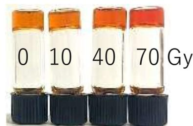
Figure 6. Images of dry dichloromethane gel of **3** after  $\gamma$  irradiation ( $[\mathbf{3}]_0 = 29.7 \text{ mM}$ ).
