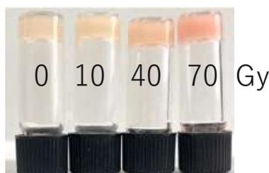
Figure 8. Image of dry dichloromethane-2 gel of **3** after  $\gamma$  irradiation ( $[\mathbf{3}]_0 = 29.7 \text{ mM}$ ,  $[\mathbf{2}]_0 = 44.2 \text{ mM}$ ).
