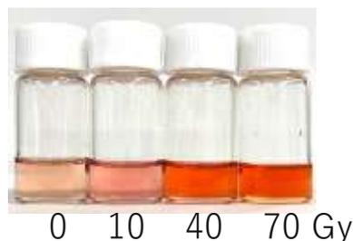
Figure 5. Images of dichloromethane solution of **3** after  $\gamma$  irradiation ( $[\mathbf{3}]_0 = 0.26 \text{ mM}$ ).
