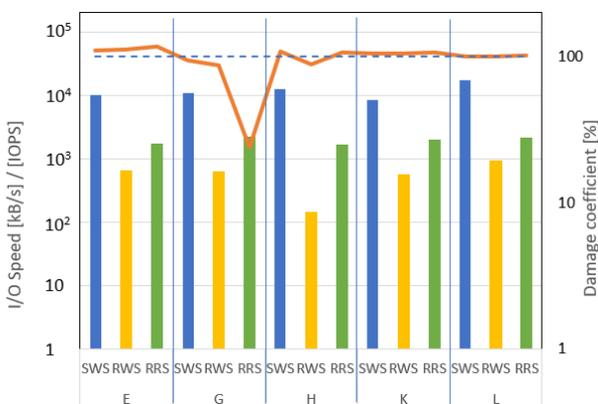
Figure 1. I/O speed of microSD cards before gamma-ray irradiation and damage coefficient after irradiation.
