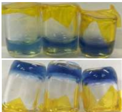
Figure 18. Images of color former 8 in \kappa -carrageenan gel containing bentonite after ^{12}\text{C}^{5+} beam irradiation (up) and one day after (down) ( [\mathbf{8}]_0 = 0.125 mM, [\text{Fe}^{2+}]_0 = 1.25 mM, [\text{Bentonite}]_0 = 0.16 g/L).
