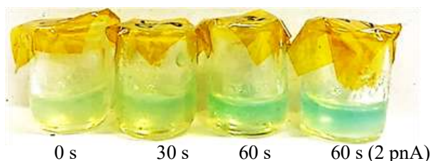
Figure 9. Images of 5a gel of 7 after ^{12}\text{C}^{5+} beam irradiation ( [\text{7}]_0 = 0.13 \text{ mM} , [\text{5a}]_0 = 5.2 \text{ mM} , [\text{Fe}^{2+}]_0 = 0.65 \text{ mM} ).
