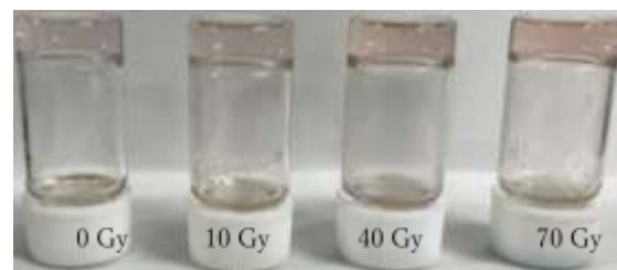
Figure 3. Images of \kappa -carrageenan gel of 3+4 after \gamma irradiation ( [3]_0 = 0.72 \text{ mM} , [4]_0 = 0.32 \text{ mM} , [\text{POD}]_0 = 0.40 \mu\text{M} , [\text{NaOH}]_0 = 10 \mu\text{M} , [\kappa\text{-carrageenan}]_0 = 15 \text{ gL}^{-1} ).
