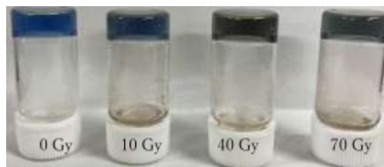
Figure 2. Images of \kappa -carrageenan gel of 1+2 after \gamma irradiation ( [1]_0 = 0.72 \text{ mM} , [2]_0 = 0.32 \text{ mM} , [\text{POD}]_0 = 0.40 \mu\text{M} , [\text{Na}_2\text{SO}_3]_0 = 0.02 \mu\text{M} , [\kappa\text{-carrageenan}]_0 = 15 \text{ gL}^{-1} ).
