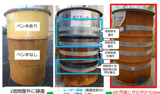
Fig. 3 A drum left for 4 months for accelerated corrosion test @ JAEA.
