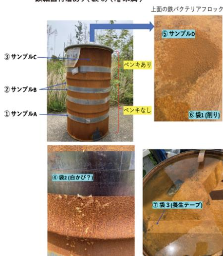
Fig.4 Details of the sampling locations from the drum can.
