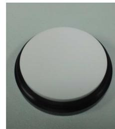
Figure 3. (upper) Spectrophotometer with integrating sphere for the spectral hemispherical reflectance measurements. (lower) Spectralon 99% reflectance standard.
