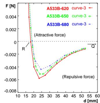
Fig. 1 : Variation of the force with different tempering temperatures
