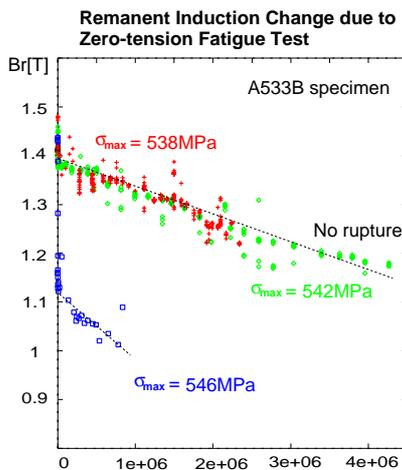
Fig. 2 : Remanent induction vs. number of fatigue cycles
